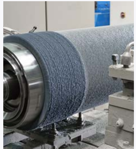
Step 2 - To achieve the best possible result, the brush surface is trimmed and processed.
