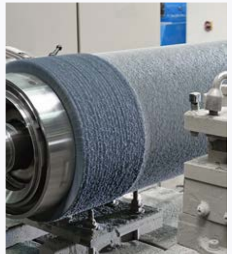
Step 2 - To achieve the best possible result, the brush surface is sheared and processed.
