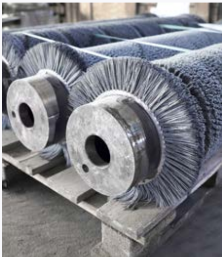
Before - the filling is worn out and needs to be refilled
