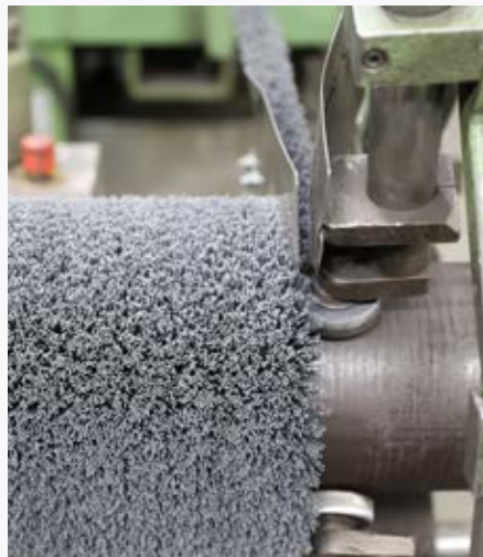
Step 1 - The used material gets completely removed and the roller is covered with new material
