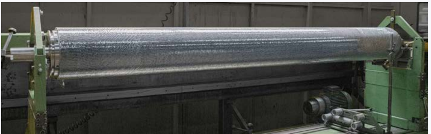
Step 3 - The brush is carefully aligned and precisely balanced to ensure optimal results.
