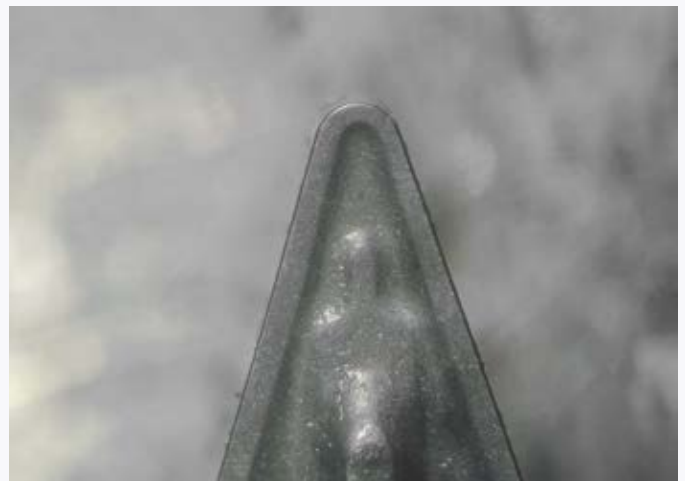
Carbide metal insert, with edge processed
