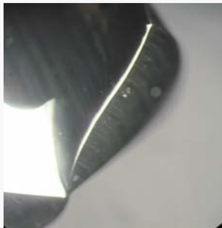
Processed with wheel brush Ø150 SIC abrasive nylon grit 180
