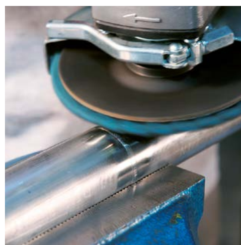
Finishing of weld seam with polishing flap wheel
