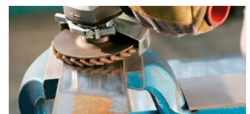
Efficient rust and scale removal
