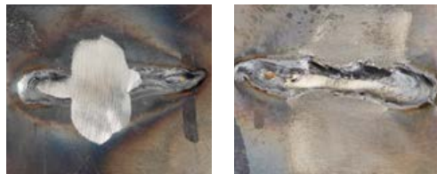
Differences in processing: On the left, processing with a grinding disc (stock removal), right with a brush (surface finishing only).
